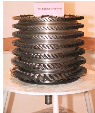
Fig. 6: Rotor of the seven-stage compressor
